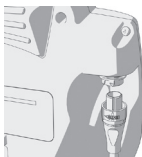
Video cable disconnected from monitor
